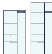
Style O2L Left: Open Shelves, Box/L-Box Right: 9" Locker 18D x 24W x 54H 18D x 24W x 62H 24D x 24W x 54H 24D x 24W x 62H
