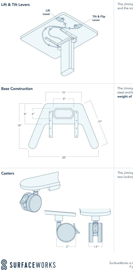
The Jimmy Table features **two adjustment levers**: The front lever controls lift and the side lever controls flip and tilt. Refer to **<u>user guide</u>** for instructions.
