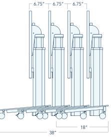
The Jimmy Table safely and easily flips down with the inclined base providing for **straight-on nesting**. Each additional nested table adds approximately 6.75" to the overall depth of all nested tables.
